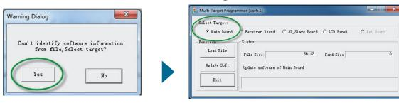
10. Click [**Update Soft**] to upload the software to the device. The software will show a progress bar.
