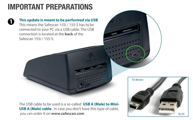
If your PC runs Windows 7 or higher, your Safescan device should automatically be recognized (as "Prolific USB-to-Serial Comm Port"). This can be checked in the Windows Device Manager.
